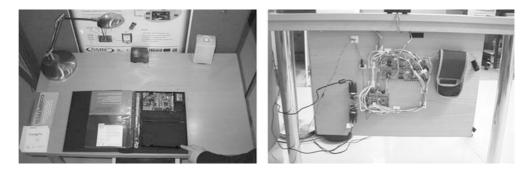
**Fig. 2** The top surface of the e-Table and the supporting circuitry underneath
